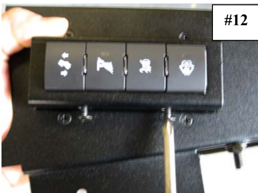
Attach switch box to console using T-20 torx screws. Do not over tighten screws. This will cause the switches to “stick” in the ON position.
